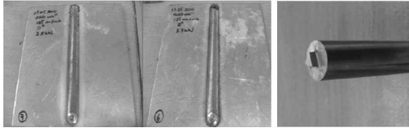
Fig. 1 General view of welded joints and tool shape
