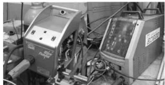
Fig. 1 Wire feeder and CO 2 welding machine
