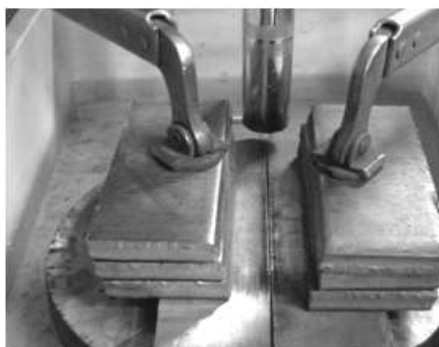
Fig. 1 Validity test of arc force(Cu plate)
