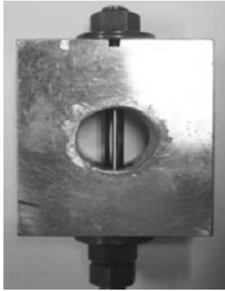
Fig. 4 Bolt tightening to the yield strength by torque wrench equipment
