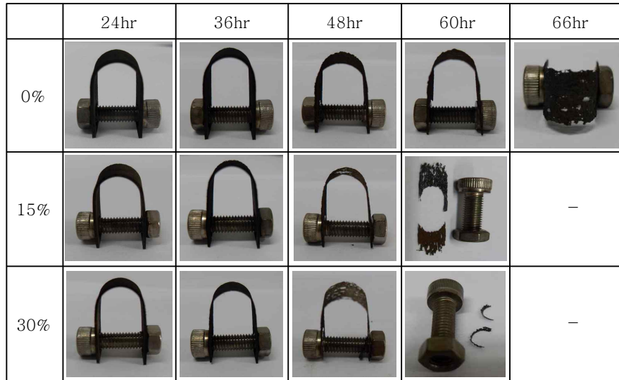
Fig. 3 Hydrogen delayed fracture for TWIP steels in 5% HCl solution using U-bending method 13)
