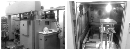
Fig. 3 Electron beam welding system used
