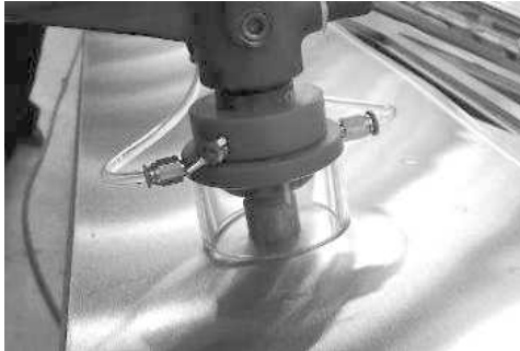
(a) Purging tool for portable spot process
