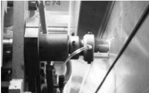
(b) Purging tool for Indirect spot process
