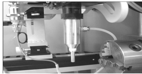
Fig. 8 Welding nozzle using assistant He gas
