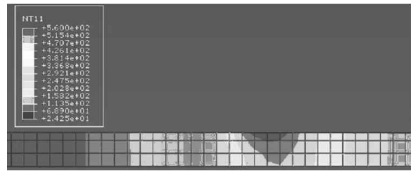
Fig. 12 Temperature field distribution at 52.51s in the section perpendicular to the weld direction when the tool is at the middle point of the plate
