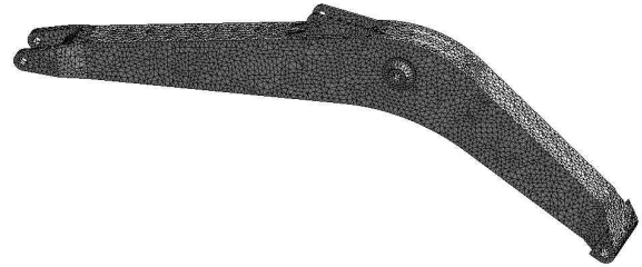
Fig. 2 Finite element model of boom structure
