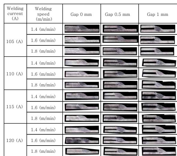
Fig. 6 Cross section according to welding conditions
