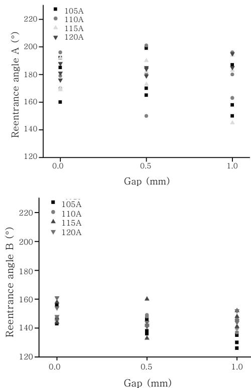
Fig. 7 Reentrance angle A, B according to welding conditions
