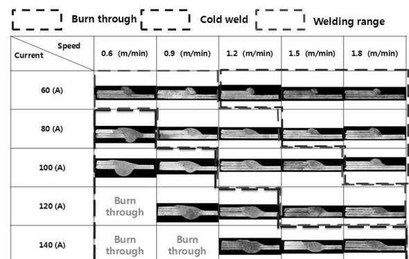
Fig. 4 Welding range at torch angle 50°
