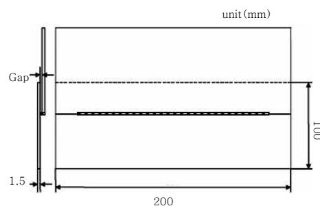
Fig. 1 Shape of welding Al 5052 specimen
