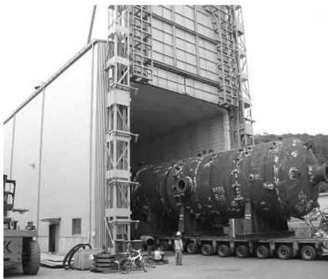
Fig. 9 Photo of large scale furnace for PWHT
