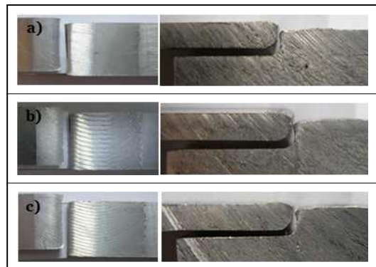
Fig. 11 Fracture appearances of A-type joint after tensile test : a) 900rpm, b) 1200rpm, c) 1500rpm(fixed 100mm/min)
