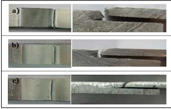
Fig. 12 Fracture appearances of R-type joint after tensile test : a) 900rpm, b) 1200rpm, c) 1500rpm(fixed 100mm/min)
