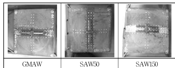
Fig. 5 Specimen appearance after 2nd CST
