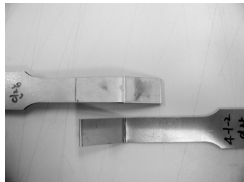
Fig. 3 Specimen after tensile-shear test
