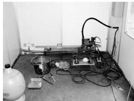
Fig. 4 Test setup equipped in the environmental chamber to keep constant temperature and humidity
