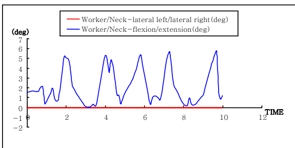
Fig. 9 Moving angle of neck after improving the overhead welding position
