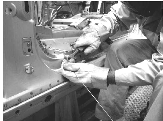
Fig. 7 Plasma-Brazing in the Automotive Industry
