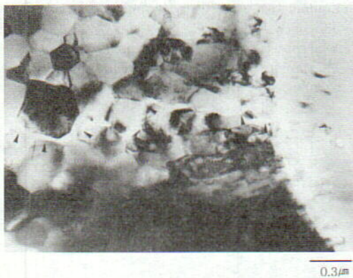
Fig. 6 Grain-boundary crack propagation in the Al 2 O 3 matrix of the 25% YSZf + Al 2 O 3 composite coating. The crack is indicated
