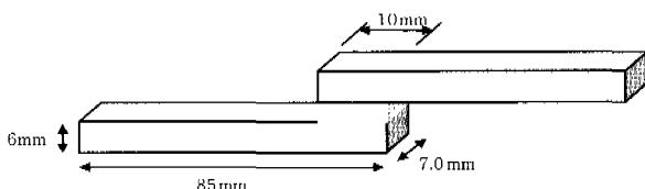
Fig. 2 Schematic of the shear tensile test specimen
