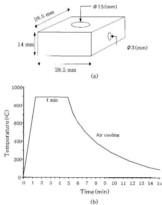
Fig. 1 Schematics of wettability test specimen and its thermal cycle
