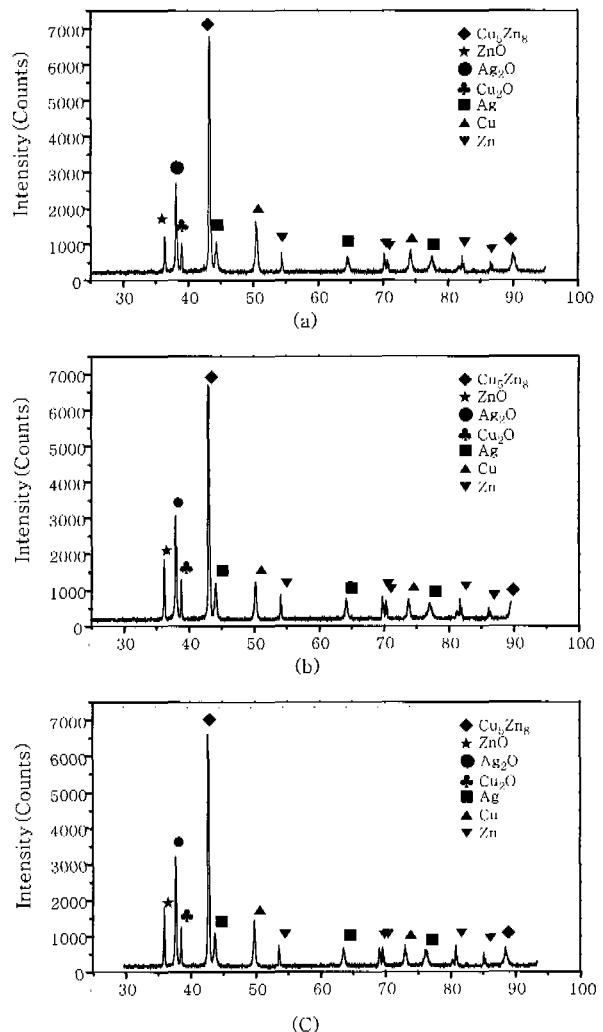
Fig. 5 X-Ray diffraction patterns of the MB-1 insert metals (a)24h (b)48h (c)72h
