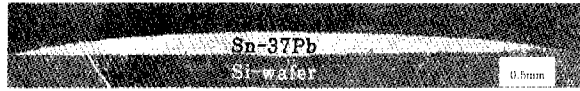
Fig. 4 Wetted state of rolled Sn-37wt%Pb solder after fluxless 1 st reflow at 230°C
