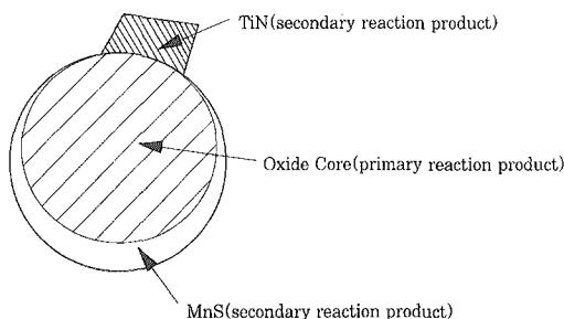
Fig. 6 Schematic diagram showing the three major constituent phases in weld metal inclusion<sup>30)</sup>.
