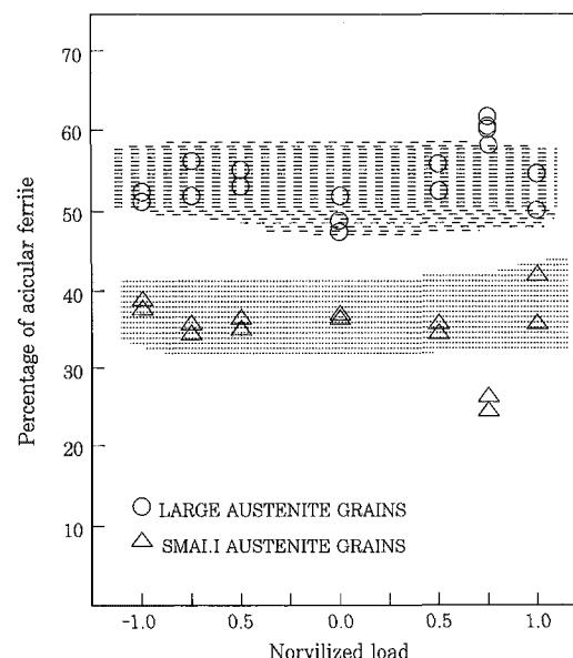
Fig. 10 The variation of acicular ferrite with the different loading conditions<sup>42</sup>.
