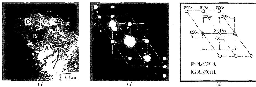
Fig. 5 TEM micrograph showing ferrite nucleation at VN precipitated on MnS: (A) MnS, (B) VN and (C) ferrite, (b) electron diffraction pattern and (c) the orientation relationship between the area B and the area C<sup>16)</sup>.
