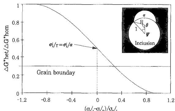
Fig. 4 Activation energy barrier of heterogeneous nucleation as a function of the difference between/inclusion and/inclusion interfacial energies per unit area of interface<sup>21)</sup>.
