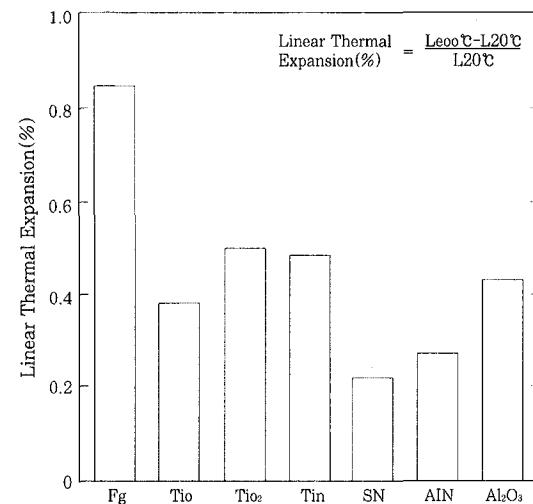
Fig. 9 Linear thermal expansion behavior of different types of non-metallic inclusions<sup>26</sup>.
