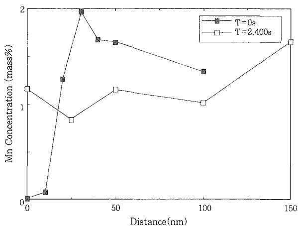
Fig. 7 Actual interfacial profiles of Mn in the as-quenched and the quenched condition after holding<sup>34)</sup>.
