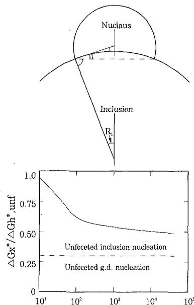
Fig. 2 Effect of inclusion size on the energy barrier for ferrite nucleation<sup>10)</sup>.
