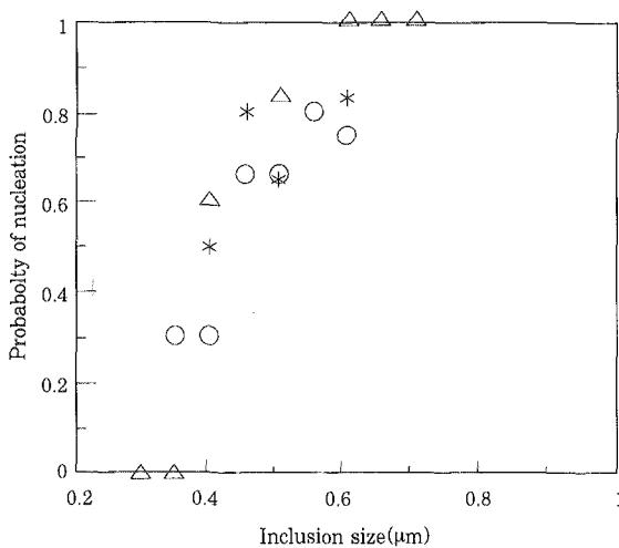
Fig. 3 Effect of inclusion size on the probability of acicular ferrite nucleation<sup>9,20)</sup>.
