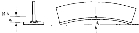
Fig. 3 Longitudinal bending deformation of built-up beam
