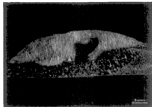
Photo. 3 Cross-section of the blowhole formed near the last stage of solidification
