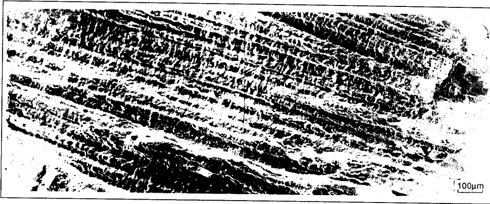
Fig. 4 SEM fractograph of a solidification crack
