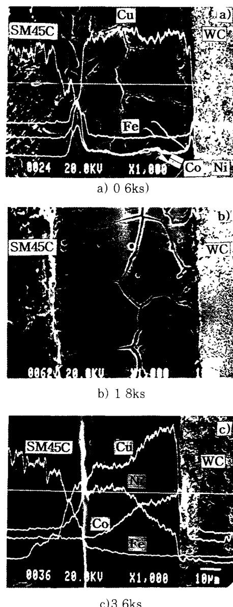
Fig.1 EPMA analysis of WC-4wt %Co/SM45C jointed at 1323K
