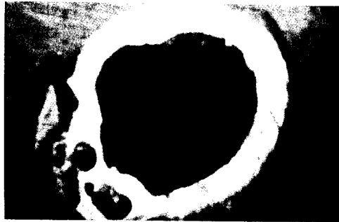
Fig. 9 Cross section of the spatter by pore escape
