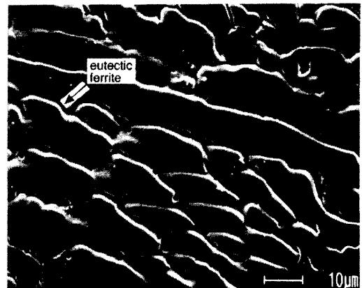
Fig. 8 Primary austenite solidification, near fusion boundary of a GTA weld in type 316L austenitic stainless steel
