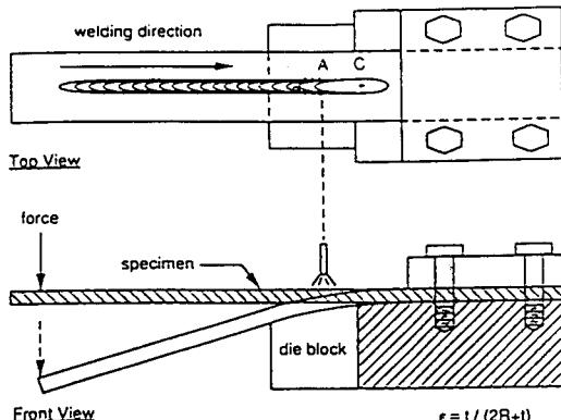
Fig. 1 Schematic of Longitudinal-Vrestraint test.
