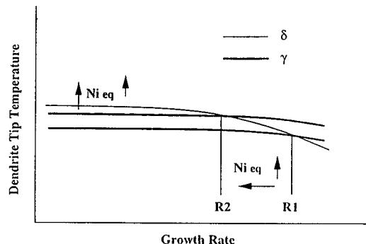
Fig. 9 Relationship between dendrite tip temperature and solidification growth rate<sup>16)</sup>.
