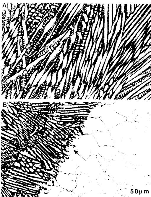
**Fig. 10** Micrographs of GTA weld in type 309S stainless steel:
