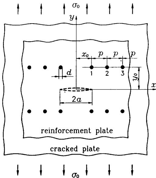
Fig. 1 Reinforced cracked plate subjected to remote uniform normal stress.
