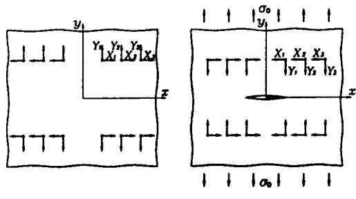
Fig. 2 Free body diagram of the reinforced cracked plate subjected to remote normal stress
