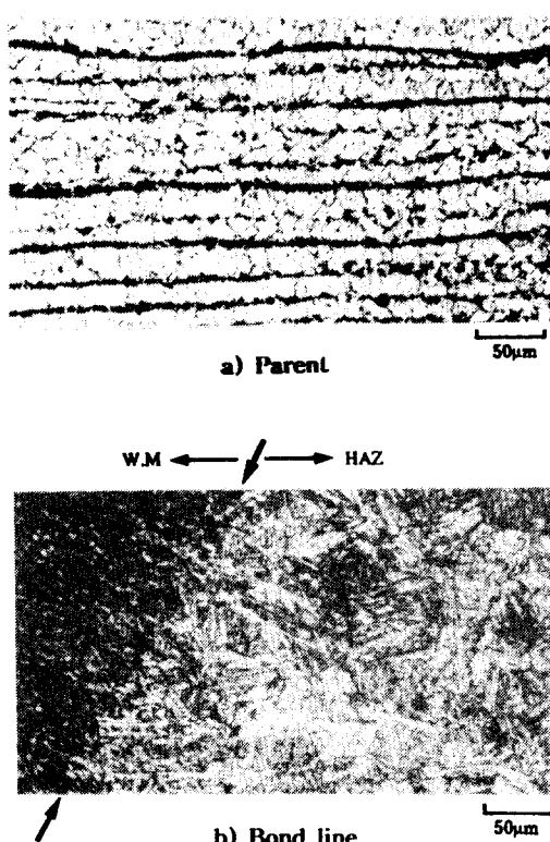
Fig. 4 Various microstructures of weld joint in HT 50 steel
