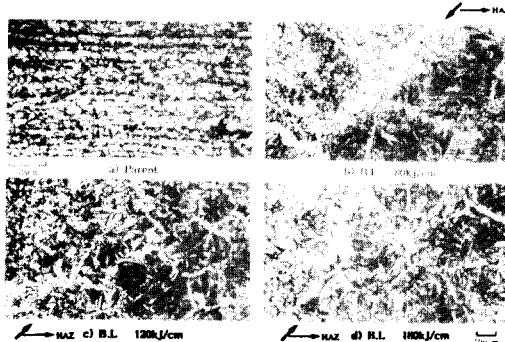
Fig. 3 Various microstructures of weld joint with weld heat input in TMCP AH36 steel
