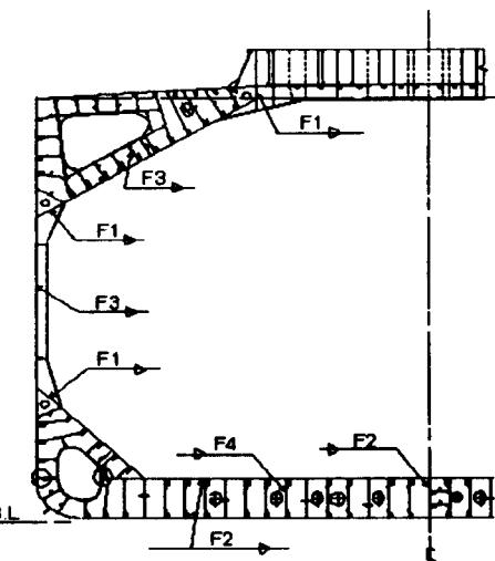
Fig. 1 Requirements of Leg length for Fillet Weld in Classification Rule (KR)
