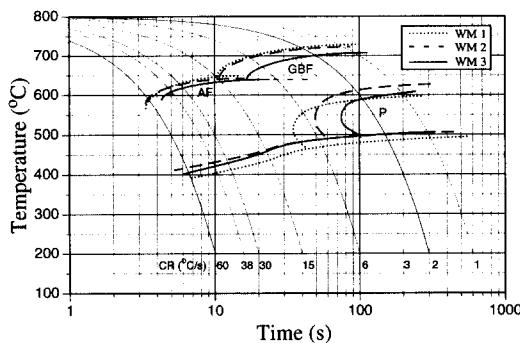
Fig. 5 Continuous cooling transformation diagrams of weld metal.
