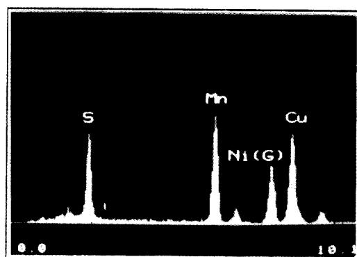
**Fig. 3** EDX spectrum of the patched-inclusion indicated by an arrow in figure 2.
