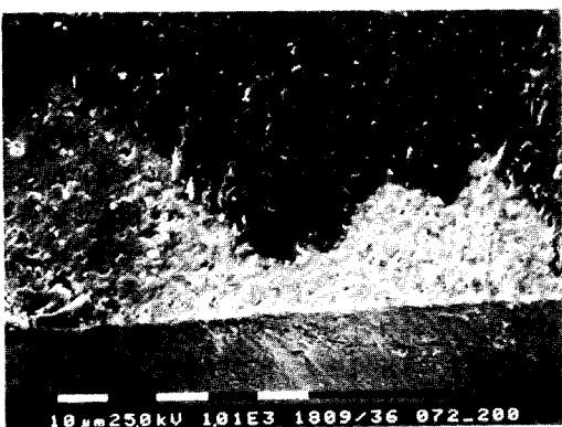
(b) fracture initiated region of the SiC/SiC joint with
