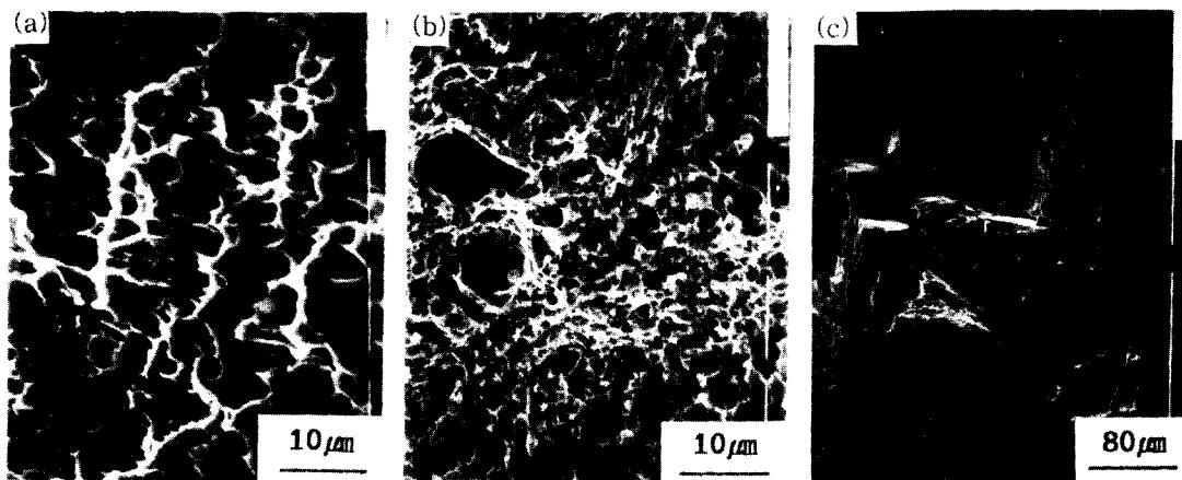
**Fig. 10** Fracture surface of broken subsize samples notched by diamond wheel.
