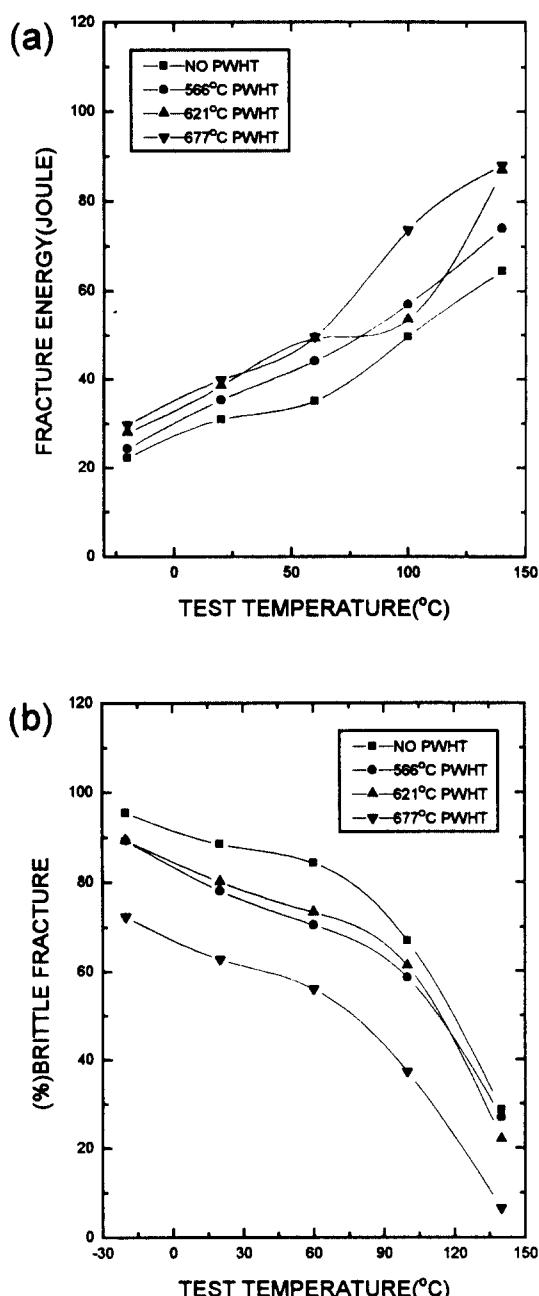
Fig. 8 Charpy V-notch impact test results of weldment.
