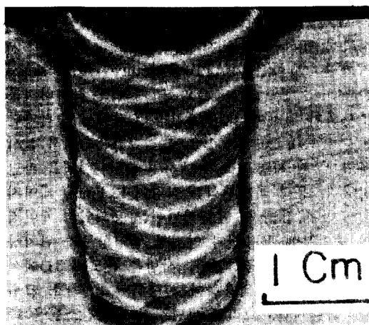
Fig. 2 Macrostructure at cross section of the weldment showing fairly uniform heat affected zone.
