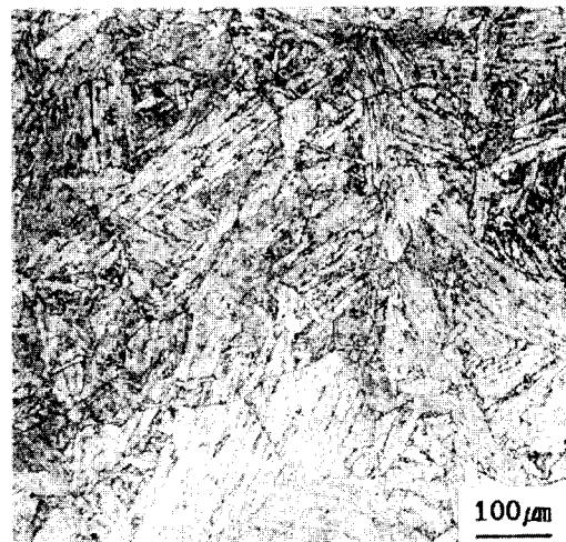
Fig. 3 Microstructure of the unaffected parent material.
