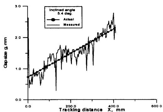
Fig. 13 Variation of gap size during visual seam tracking
