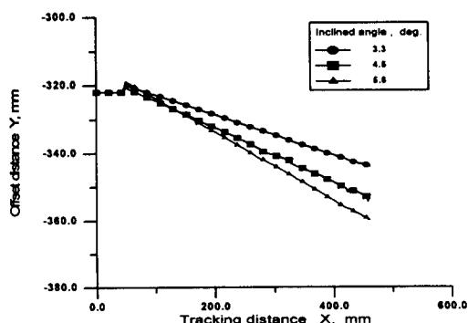
**Fig. 10** Y-axis locus of torch during visual gap tracking without welding
