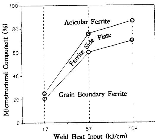
Fig. 2 Effect of weld heat input on microstructure of deposit weld metal.
