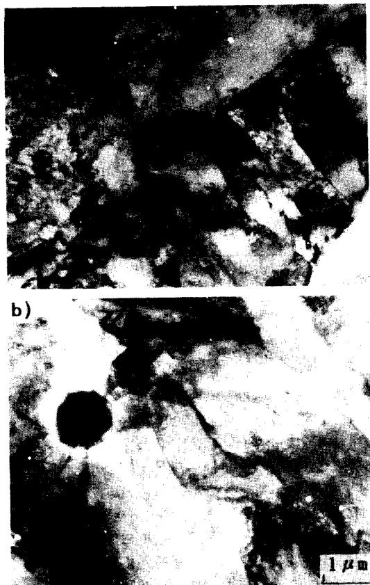
Fig. 12 (a) Fine lath ferrite developing along grain boundary ferrite
