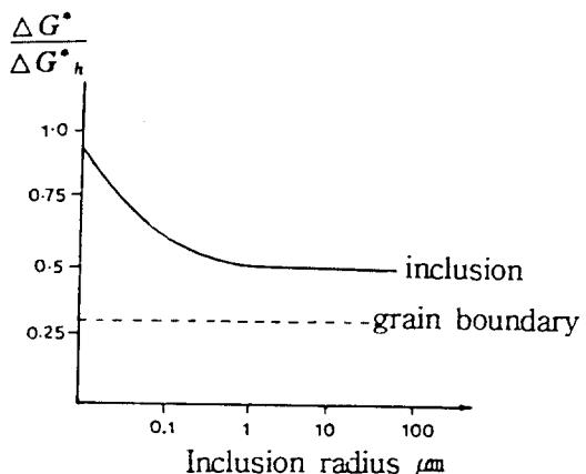
Fig. 11 Plot of a normalized energy barrier to nucleation of ferrite at an inclusion and at a grain boundary.
