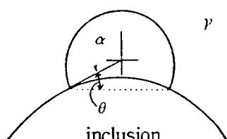
Fig. 10 Nucleation of a spherical nucleus of ferrite at an inclusion in the austenite.
