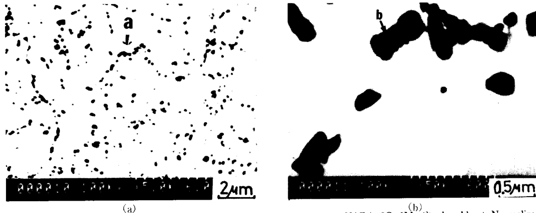
Photo. 7 Scanning Transmission Electron Micrographs of Base Metal near HAZ in 9Cr-1Mo Steel weldmet, Normalized, PWHT 730°C×1hr, Angle-cut section.
