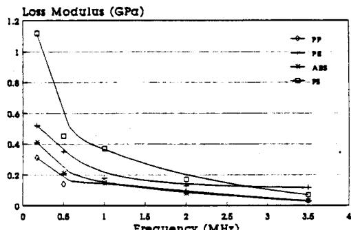
**Fig. 7** Effect of frequency on the loss modulus
