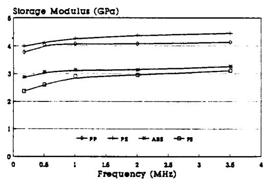
**Fig. 6** Effect of frequency on the storage modulus
