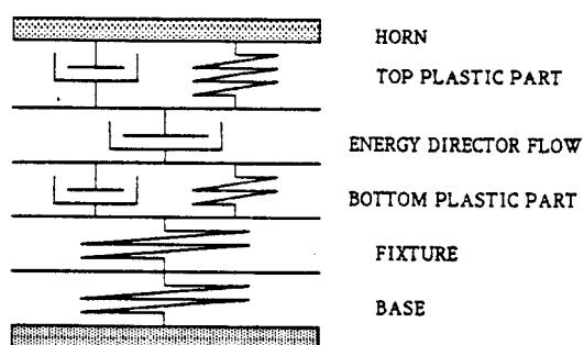
Fig. 1 Lumped-parameter model for ultrasonic welder
