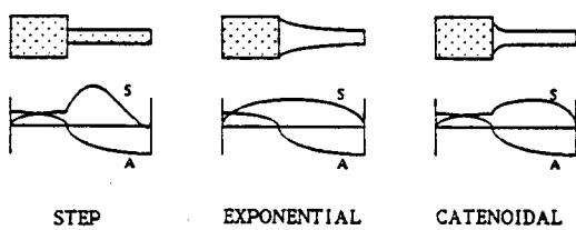
**Fig. 4** Examples of horn geometries with the resulting Stress(S), and displacement amplitude(A) distributions
