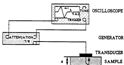
Fig. 3 Measurement of sound velocity and attenuation
