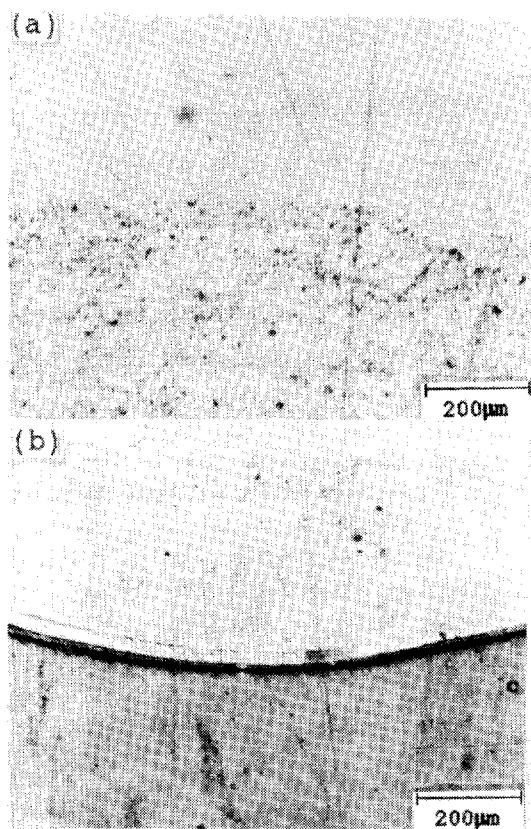
**Photo.3** Micrographs of weld intergace(ABS-PS, ABS-PP)
