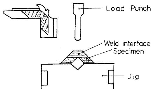
Fig. 6 Bending test specimen of friction weld and jig
