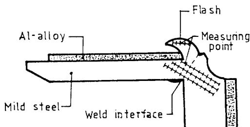
Fig. 5 Hardness test specimen of friction weld
