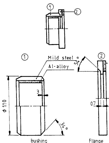
Fig. 4 Specimen for friction welding test
