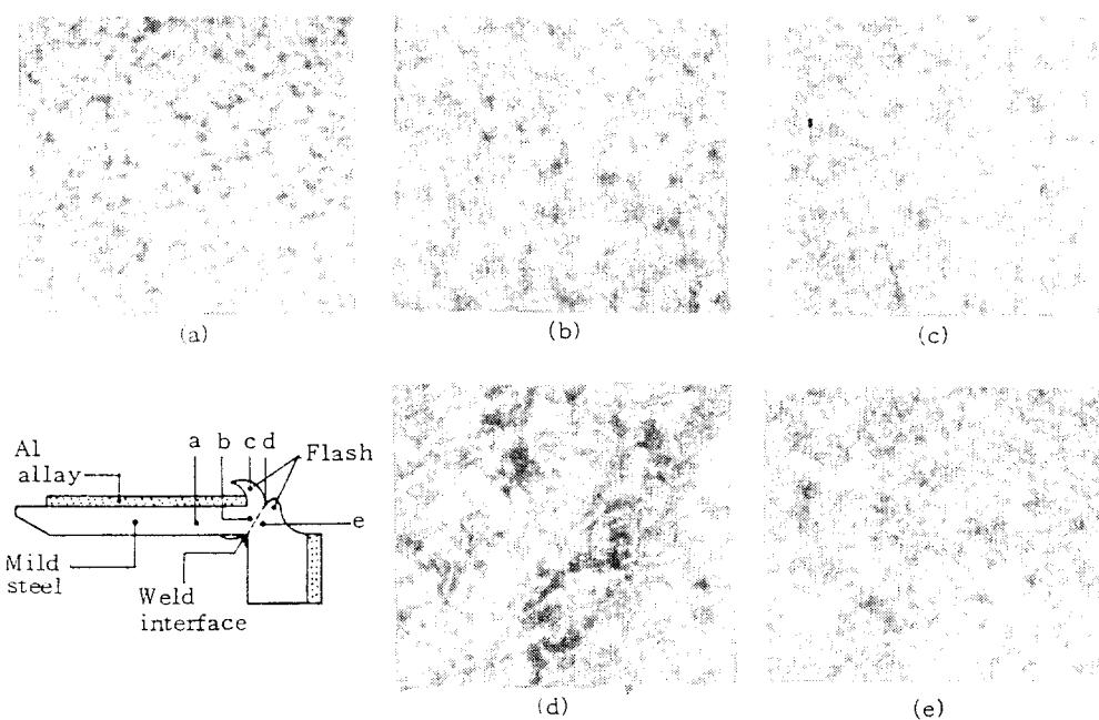
**Photo. 1** Microstructures of friction weld joint (low-carbon steel)
