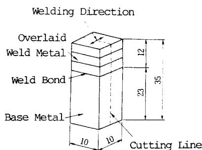
Fig. 1 Dimension of test specimen(mm)
