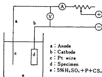
Fig. 3 The electrochemical circuit for the hydrogenation
