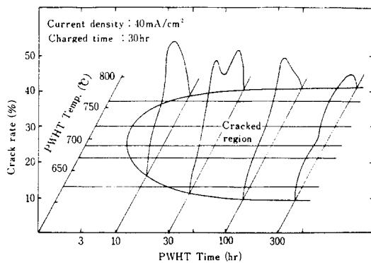
Fig. 7 Relation between PWHT condition and crack rate
