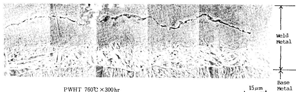
Photo. 6 Typical hydrogen embrittlement crack under non load
