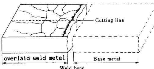
Fig. 2 Strauss test specimens
