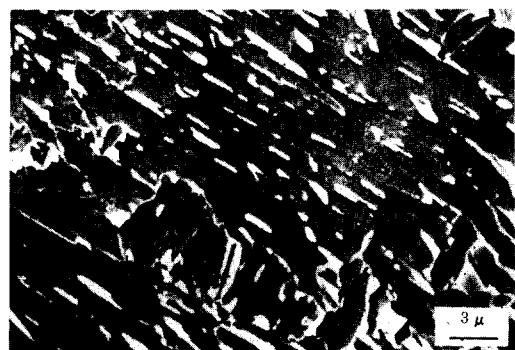
**Photo. 4** Scanning electron micrograph in the simulated ICRCG HAZ prepared by the 2-stage electrolytic etching technique<sup>12)</sup> to observe M-A constituent
