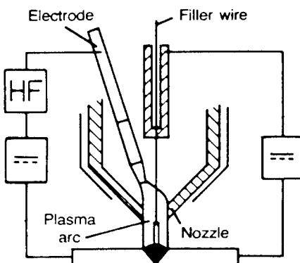
Fig. 7. Schematic diagram of a plasma-GMAW
