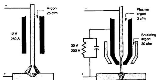
**Fig. 1.** Arc column shape for GTAW and PAW
