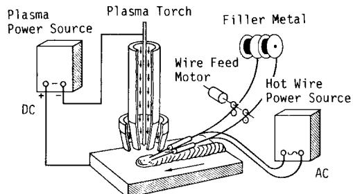
Fig. 9. Schematic diagram of plasma hot-wire overlay welding
