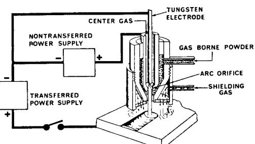
Fig. 8. Schematic diagram of plasma powder overlay welding
