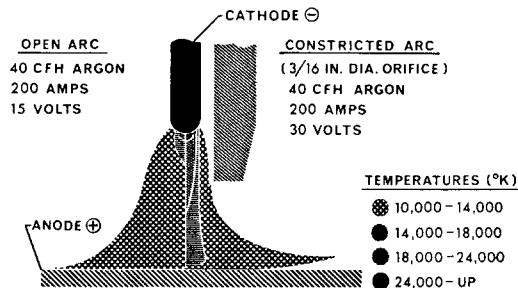
Fig. 2. Effect of arc constriction on temperature in arc.
