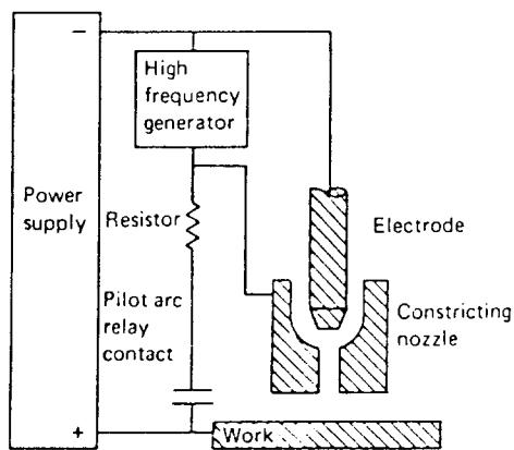
Fig. 10. Basic plasma arc cutting circuitry
