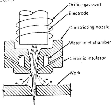
Fig. 11. Water injection plasma arc cutting arrangement
