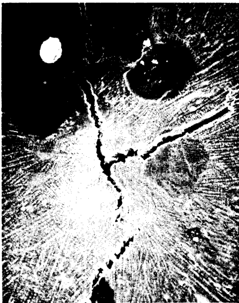
Fig. 9. Appearance of SK-5/PBS plates(0.2/0.4mm) spot-welded under laser power 30J/pulse, pulse duration 9ms.
