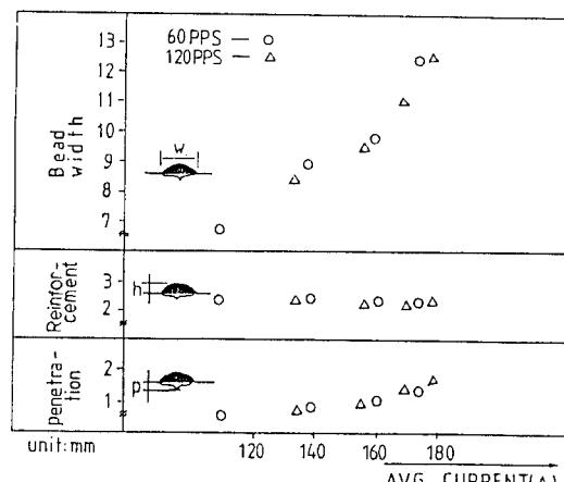
Fig. 6. Effect of average current on bead shapes.
