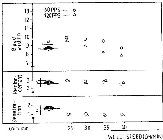
Fig. 7. Effect of weld speed on bead shape
