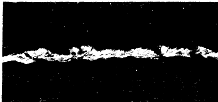
Welding Condition: 140Amp - 25V - 30Cm/m
