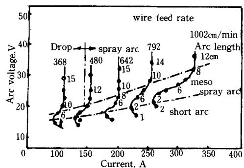
Fig. 9. Voltage/Current relationships for various wire feed speed in MIG-welding aluminum. Material: 1.6mm diameter A5183 wire in argon.
