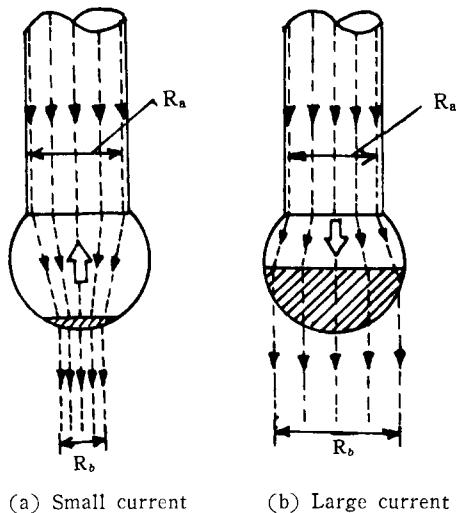
Fig. 21. Effect of arc size on droplet detachment force; active area and direction of axial force
