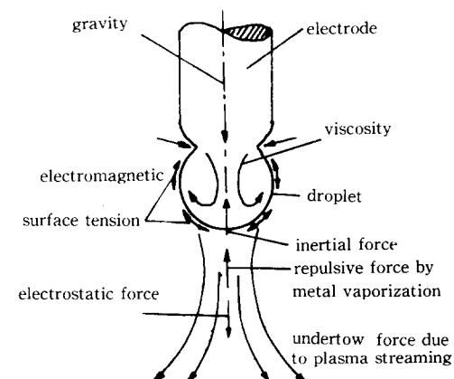
**Fig. 16.** Different forces acting on metal transfer
