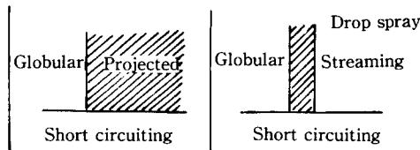
Fig. 6. Schematic diagram of relationships between metal transfer, welding current, and arc voltage
