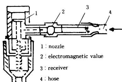
Fig. 25. Diagram of deivece for the short-term increase in velocity of the shielding gas
