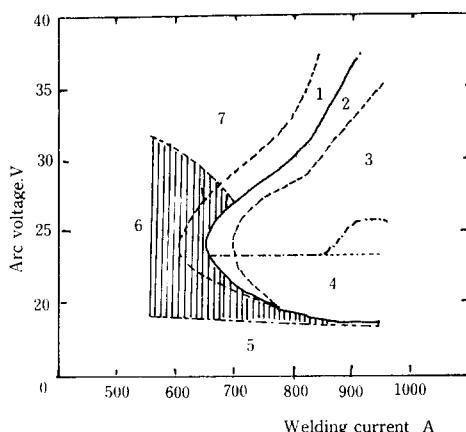
**Fig. 11.** Relationship between droplet transfer, welding current, and arc voltage. Shielding gas —Ar+25%CO<sub>2</sub>; welding speed —60 mm/min; L—20mm. 1—globular+projected; 2—projected+streaming; 3—streaming; 4—instant short circuiting; 5—stubbying; 6—short circuiting; 7—globular
