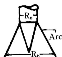
Fig. 20.\* Schematic of melting and tip formation
