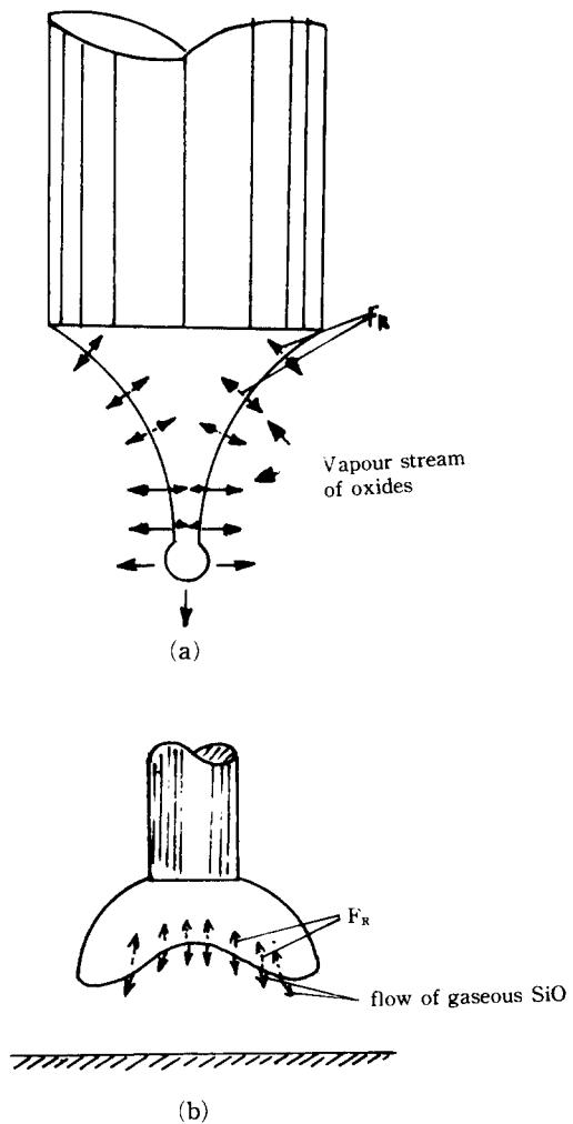
Fig. 23. Schermatic of molten metal on electrode tip; (a) streaming (b) repelled conditions
