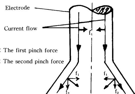
Fig. 19. Two types of electromagnetic force
