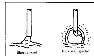
Fig. 5. Schematic representation of metal transfers
