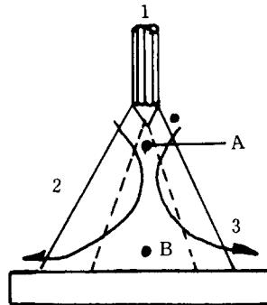
Fig. 22. Schematic of plasma gas flow generation and measurement of dynamic pressure
