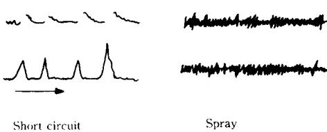
Fig. 4. Typical oscillograms of different type metal transfer mode
