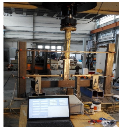
Fig. 12 Compressive test configuration
