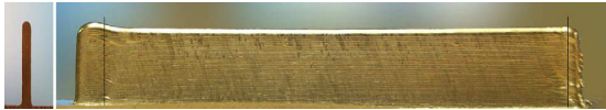
Fig. 6 Multi-layered single bead wall deposited with automatic process control (The length of the wall: 215mm) 18)
