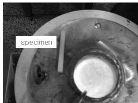
Fig. 2 Salt bath and specimen
