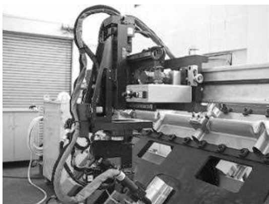
Fig. 3 Carriage machinery part of automatic welding system
