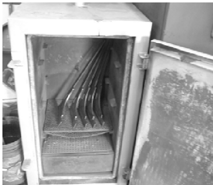
Photo 2 Furnace for PWHT of test specimens
